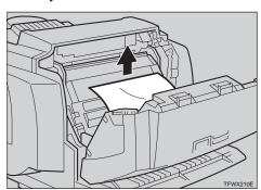
When the misfed paper is in the main section of the photoconductor unit, turn the dial downward then remove it.
